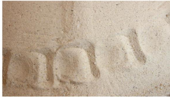
Fig. 8. Grouser-bladder contact tread marks during inflation tests.
